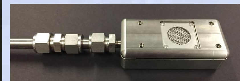
Downhole Fluids Sensor (DFS) Alpha Prototype sensor head
