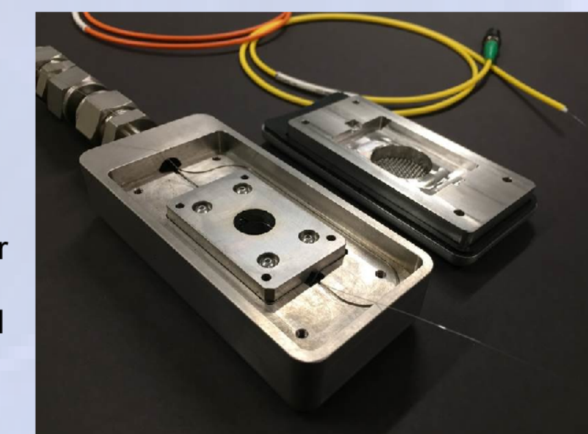
Downhole Fluids Sensor (DFS) Alpha Prototype sensor head
